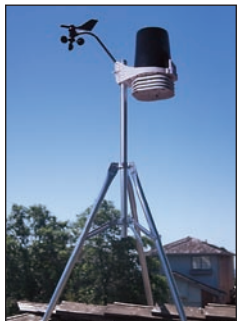
Use our optional tripod to mount the integrated sensor suite on a rooftop ...
