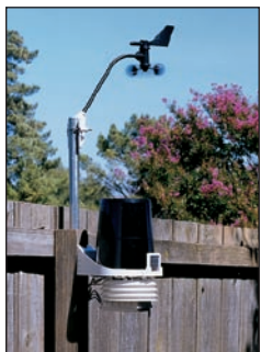
Separate the anemometer from the rain collector to mount it on a fence post up to 40' (12 m) away...
